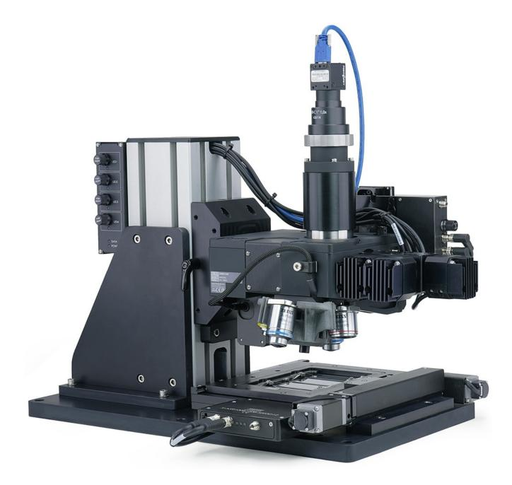
• Motorized XY and Z-focus movement, filter cube and objective changes allow fully automated whole slide imaging
