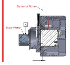
Optical distance from Input plane  $\boxed{\mathsf{A}}$  to Detecor Plane: 49  $\pm$  0.5
