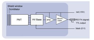
The figure above illustrates a block diagram of the internal structure of PDM03-9107-PD. It is integrated with a shield window, plastic scintillator, high performance photomultiplier, high voltage power supply incorporating voltage divider and signal processing electronics.
