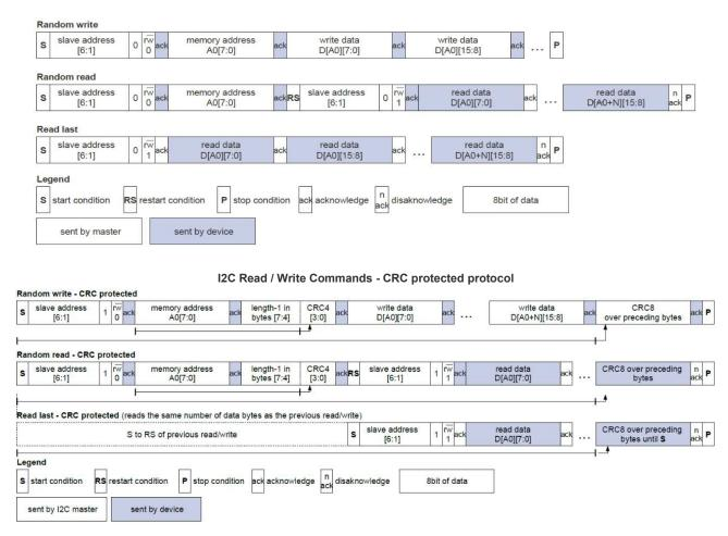
The memory address field sets the byte address of the first memory location to be read from or written to. Only 16-bit-word aligned reads/writes are supported, i.e. the LSB of memory address has to be zero always. The read/write data is transferred MSB first, low byte before high byte.
