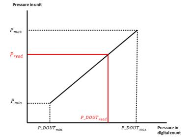
For example, the  $P_{min}$  and  $P_{max}$  for the sensor are specified as -15 psi and +15 psi. The  $DOUT_{min}$  and  $DOUT_{max}$  are 26214 and +26214. So,
