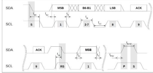
I<sup>2</sup>C Interface Timing Diagram:
